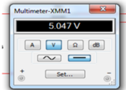
Figure 37, Output voltage of rectifier for turn ratio of 17:1
